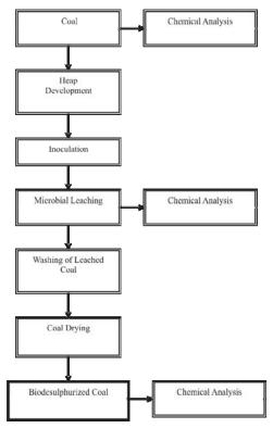
Figure - 4: Concept Outline for Heap Biodesulphurization
