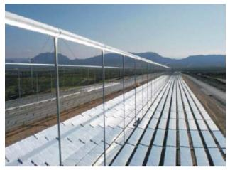
Figure - 5: A Fresnel Concentrator in Australia
