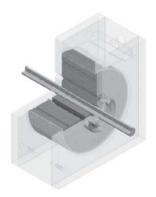
Figure - 2: Tesla Turbine
