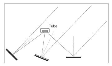
Figure-1: A Sectional View of Fresnel Mirror Arrangement
