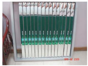
Figure - 3: Fresnel Mirror Concentrator being investigated in R&D Lab at CIIT (The camera is right above the object)
