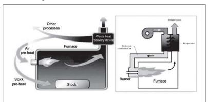
Figure - 2: Heat Recovery System for Energy-Conservation
