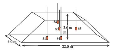
Figure - 5: Schematic Diagram of Coal Heap Established for Biodesulphurization. Heap Dimensions and Location of Temperature Sensors (S1, S2, S3, S4 & S5) inside the Heap
